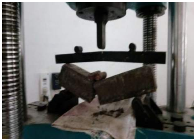
Figure 5: Flexural test of unreinforced concrete beams under Universal testing machine.
