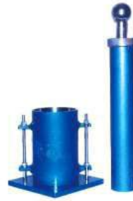
Figure 4 Standard Proctor test Apparatus
