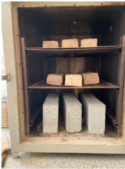
Fig.3 Block Density Test
